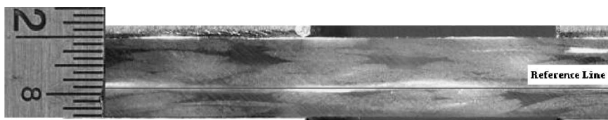
Fig. 8 Microscopic image of the axial tow undulations in a glass 2DTBC specimen: 4.93 mm (0.194 in.) thickness with 0.15–0.22-mm undulation.
