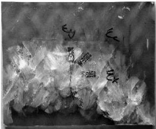
Fig. 11 Typical tow buckling phenomenon seen in compression tests; whitening of matrix due to distributed matrix cracking and fiber/matrix debonding.
